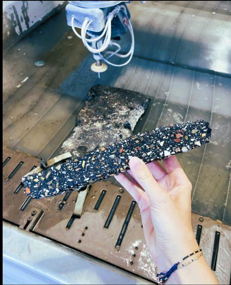
The cuts through the amorphous chunks, which were first made with a water jet cutting machine and then with a wet saw, also revealed aesthetic, terrazzo-like qualities.
