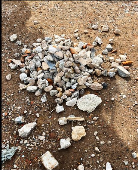
Regardless of the existing potential in terms of size, colour and shape, the construction waste is downgraded by crushing and can only be used as filling material such as gravel or sand.
